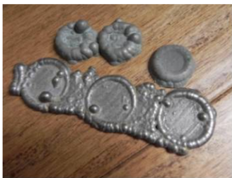
99.99% Electrolytic Nickel an Alloy Used in Austenitic Stainless Steel
