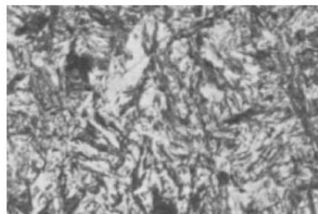
Quench Hardened but Brittle Steel HRc 65 (martensite)
